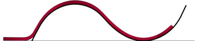
If you want your project to slump evenly on the mold, you must elevate one end to get the glass to drop evenly. Kiln posts or bricks work well to elevate the mold.
